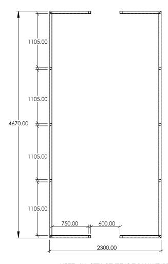
NOTE -ALL STRUCTURE IS FULLY WELDED WITH A NOMINAL FILLET RADIUS OF 5mm.
