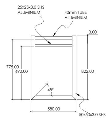
NOTE -STRUCTURE IS TO BE FULLY WELDED. HOLES ARE TO BE DRILLED ON UNDERSIDE OF MEMBERS TO ALLOW FOR WATER AND MOISTURE TO ESCAPE.
