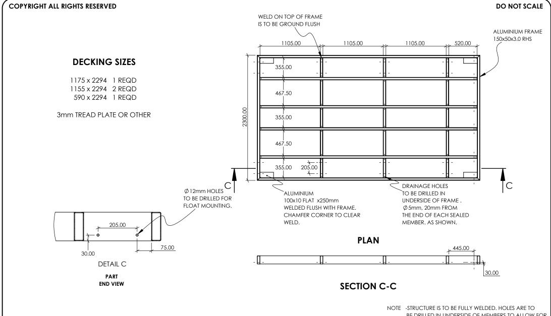
APPROX. DECK AREA - 11.5m<sup>2</sup> APPROX. FRAME WEIGHT - 110kg FLOATS NOT INCLUDED NOTE -STRUCTURE IS TO BE FULLY WELDED. HOLES ARE TO BE DRILLED IN UNDERSIDE OF MEMBERS TO ALLOW FOR WATER AND MOISTURE TO ESCAPE.
